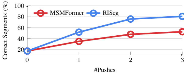
Fig. 5: Percentage of objects correctly segmented as measured by the Overlap F-measure \geq 75\% .
