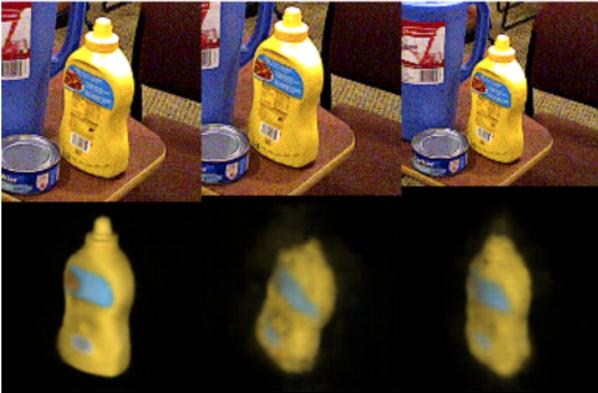
Fig. 5. Visualization of reconstruction of the RoIs from auto-encoder. Left is the ground truth RoI. The other two columns show the reconstruction with shifting and scale change. As it is shown, the reconstruction quality degrades with deviations from the ground truth RoI. In this example, the similarity score drops from 0.91 to 0.62 and 0.72 with the deviations respectively. This property makes the auto-encoder a suitable choice for computing the observation likelihood.
