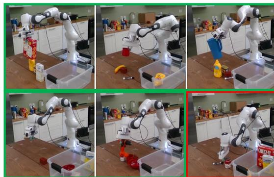
Fig. 8: Grasping performed in real cluttered environments. Here we show 5 successful and 1 failed trial on grasping YCB objects.
