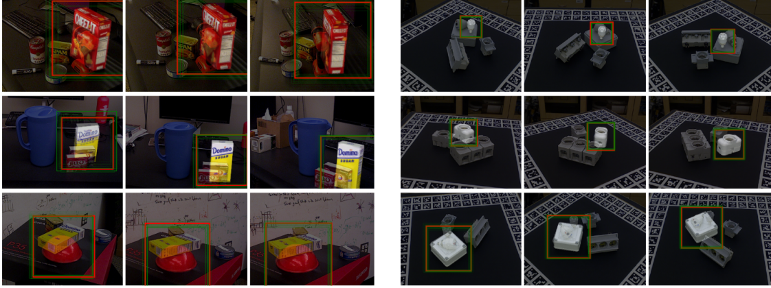
Fig. 7. Visualization of estimated poses on the YCB Video dataset (left) and T-LESS dataset (right). Ground truth bounding boxes are red, green bounding boxes are particle RoIs, and the object models are superimposed on the images at the pose estimated by PoseRBPF.
