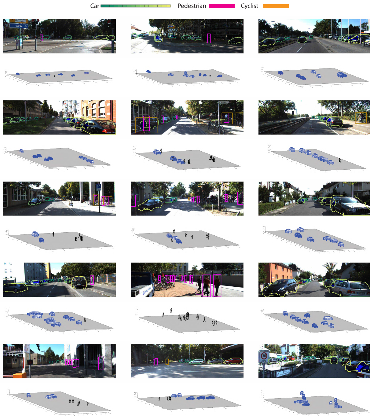
Figure 4. 2D detection and 3D localization results on the KITTI test set. Detections with scores larger than 0.5 are shown. Blue regions in the images are the estimated occluded areas.
