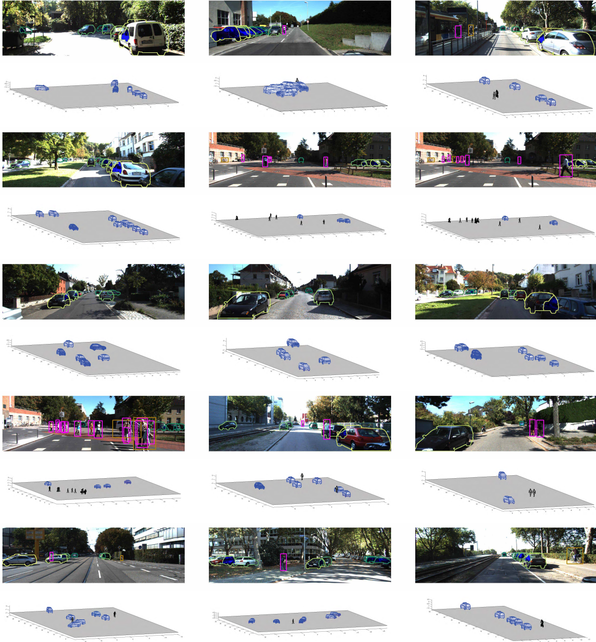
Figure 1. 2D detection and 3D localization results on the KITTI test set. Detections with scores larger than 0.5 are shown. Blue regions in the images are the estimated occluded areas.
