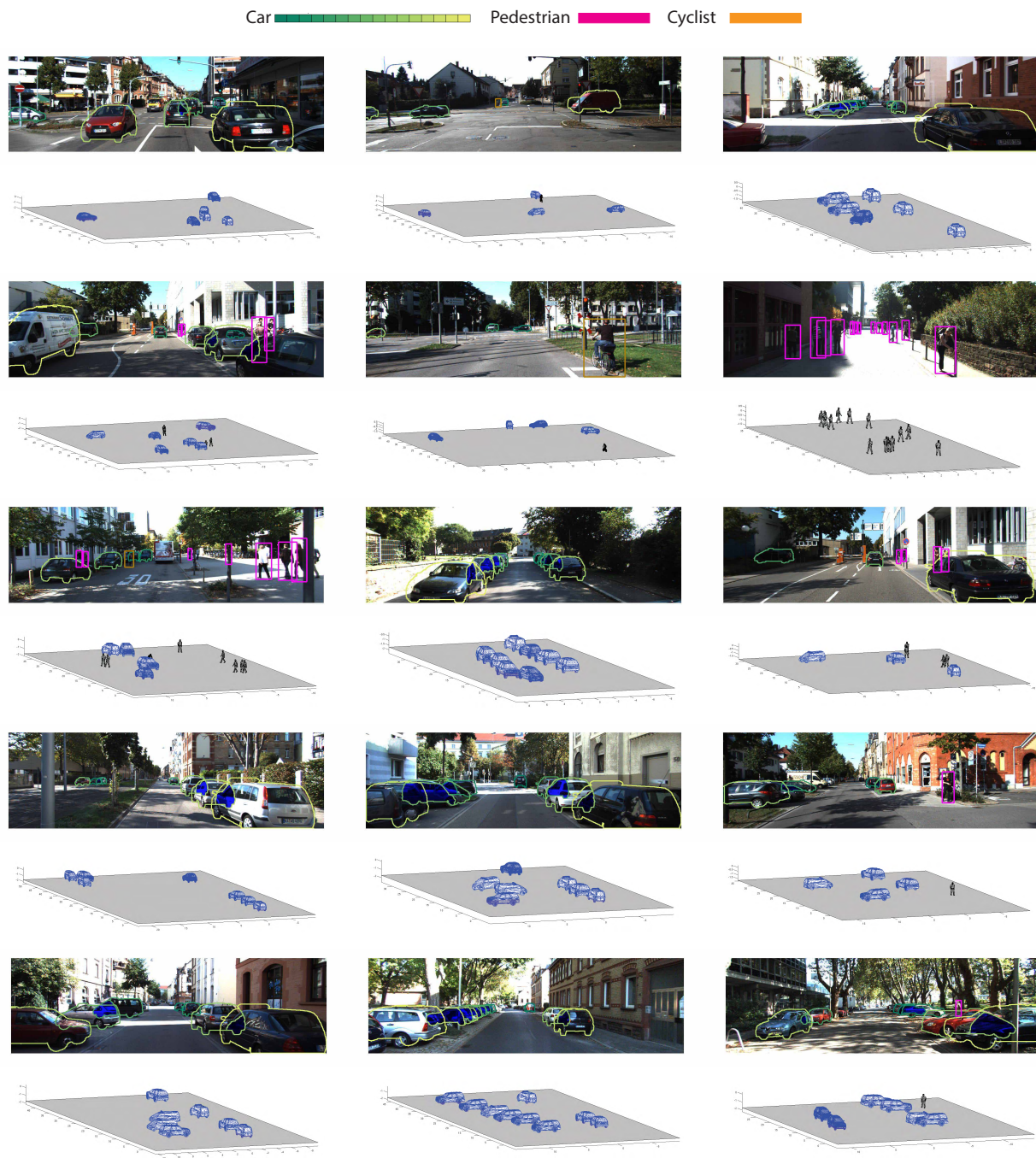
Figure 3. 2D detection and 3D localization results on the KITTI test set. Detections with scores larger than 0.5 are shown. Blue regions in the images are the estimated occluded areas.
