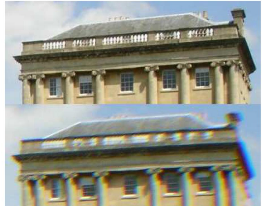
Figure 4.18: The upper image is properly focused whereas the lower image suffers from chromatic aberration. (Figure by Stan Zurek, license CC-BY-SA-2.5.)
