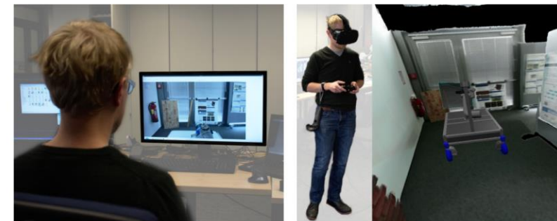
Fig. 5. Teleoperation experiment. Left: Baseline experiment with wide-angle camera feed. Right: Teleoperation using the proposed VR system.
