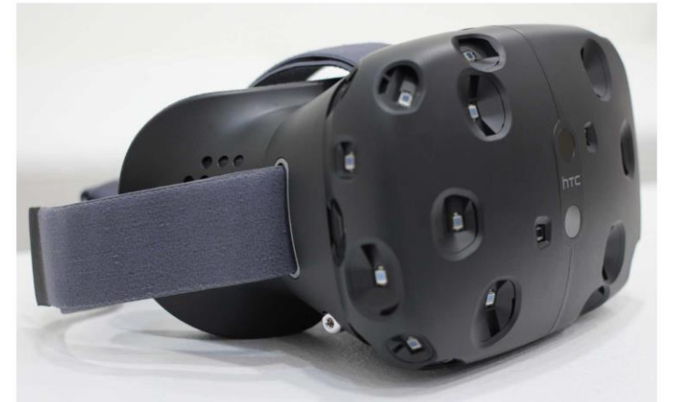
Photodiodes in pockets on the front of the headset detect the incident IR light
