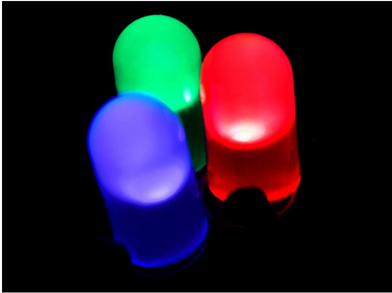
RGB LEDs: emit lights when current flows through
