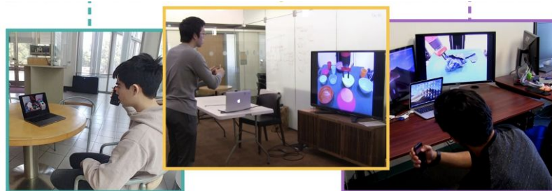
Fig. 1: Collecting data on physical robot arms with the RoboTurk platform. To collect task demonstrations, users connect to our platform from remote locations using a web browser and use their smartphone as a motion controller to move the physical robot arm in free space. Users are provided a video stream of the robot workspace in their web browser.
