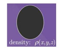
$$\mathcal{I}_{xx} = \int_{\mathcal{B}} (y^2 + z^2) \rho(x, y, z) \, dV \qquad \mathcal{I}_{xy} = -\int_{\mathcal{B}} xy \rho(x, y, z) \, dV
