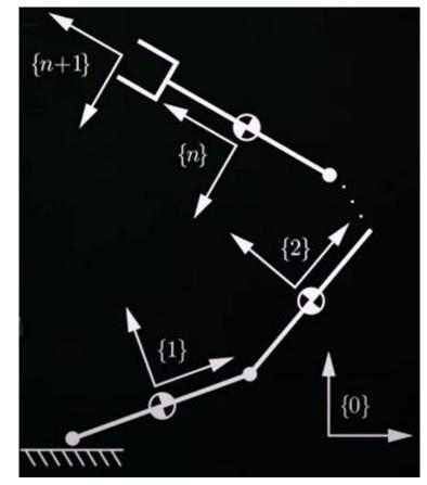
• Screw axis for joint i in link frame {i}  $A_i$  , in space frame {0}  $S_i$
