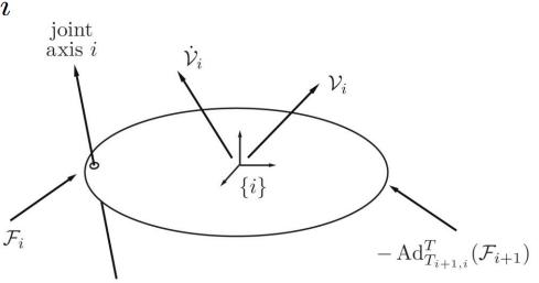
• Wrench on link i from joint i and joint i+1
