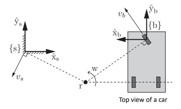
Rotation can cause linear velocity
